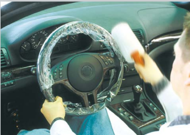
Disposable steering wheel and gear shift cover (O/N D-L 42) for steering wheels of both passenger cars and lorries, adhesive polyethylene foil with handle, for about 250 applications.
